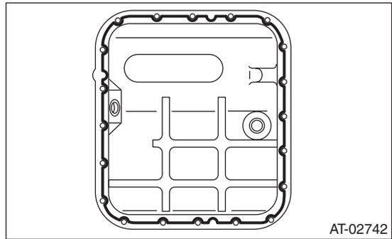
6) Apply liquid gasket fully to three holes other than screw holes on transmission case.
