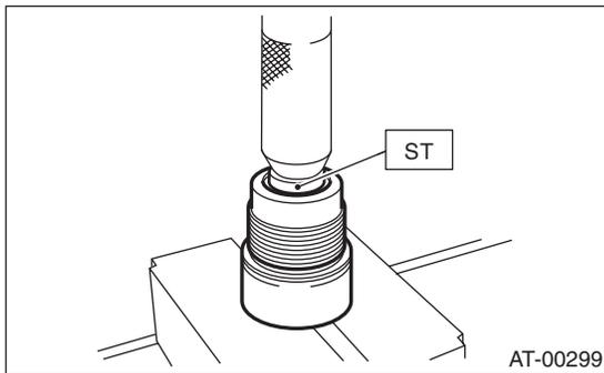
2) Apply vaseline to the groove of the inner race and to the seal ring.
