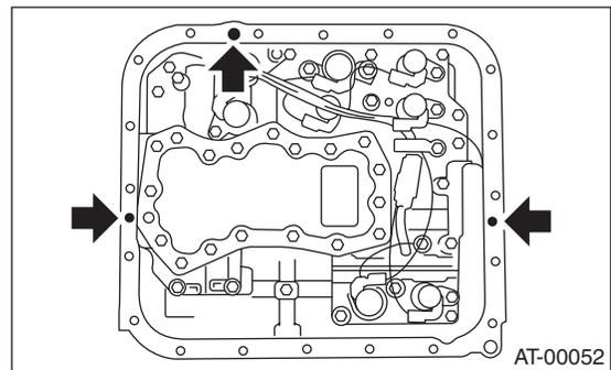
7) Install the oil pan by equally tightening the bolts.
