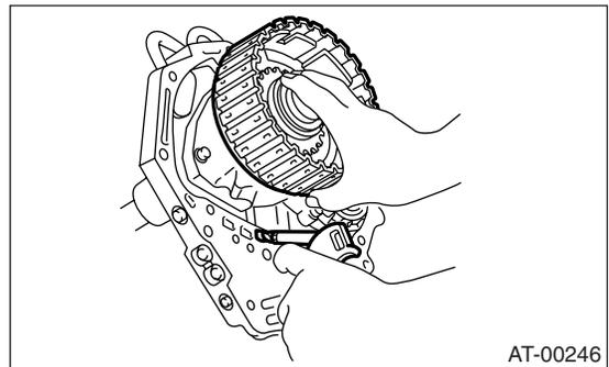
(4) Measure the clearance between the retaining plate and snap ring. (High clutch) At this time, do not press down retaining plate.
