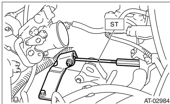
16) Remove the bolt which holds the upper side of transmission to engine.
