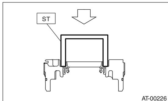
3) Apply gear oil to new O-ring and install it.
