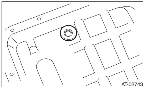
6) Apply proper amount of liquid gasket to the entire oil pan mating surface.
