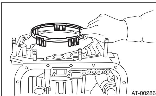
21) Position snap ring in transmission. Using ST, press the snap ring into place.
