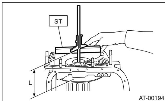
2) Using the ST, measure the distance from the oil pump housing mating surface to the end surface of ST.
