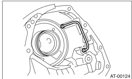
4) Apply ATF to new O-ring and install the test plug.
