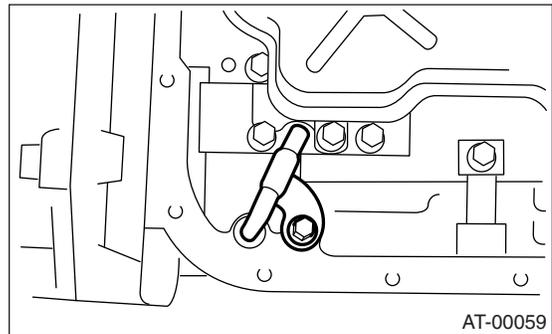
13) Remove the control valve body.
