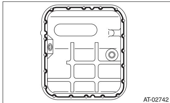
5) Apply liquid gasket fully to three holes other than screw holes on transmission case.
