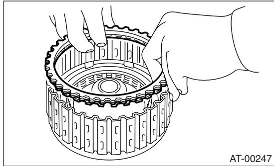
(2) Apply compressed air intermittently to check for operation.
