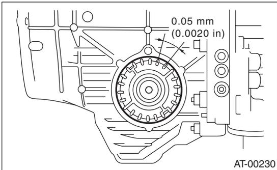
8) Turn the drive pinion several rotations with ST1 and check to see if the backlash is within the standard value with ST2, ST3, ST4 and ST5.
