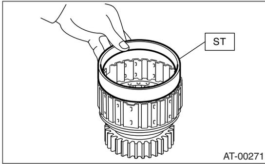
5) Set the cover on the piston with a press using ST1 and ST2, and attach the snap ring. At this time, be careful not to fold cover seal during installation.
