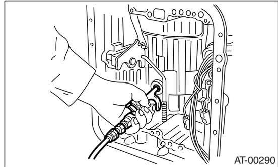
(10) Measure and record the clearance "B" between the retaining plate and snap ring.
