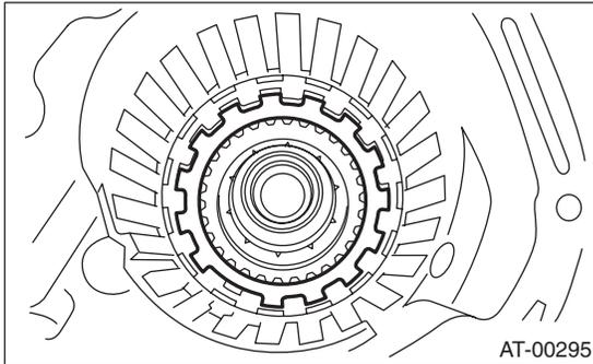
25) Turn the transmission case upside down, and then take out the socket bolts while holding the one-way clutch inner race with hand.
