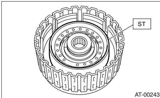
6) Avoid folding the high clutch piston seal, when installing the cover to high clutch piston.
