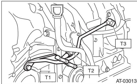
2) Install ATF cooler pipe to frame.
