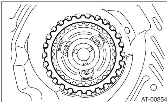
(8) Install a new 2-4 brake oil seal to transmission case.
