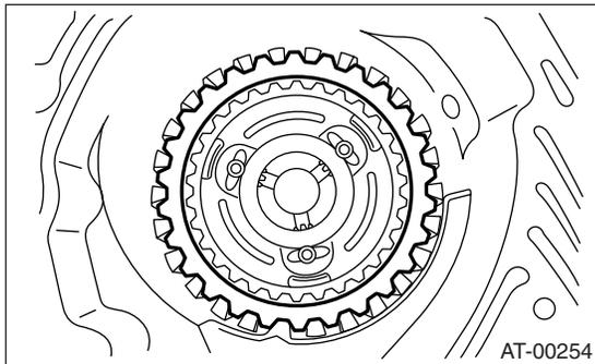
17) Take out the thrust needle bearing, planetary gear assembly and the low clutch assembly.
