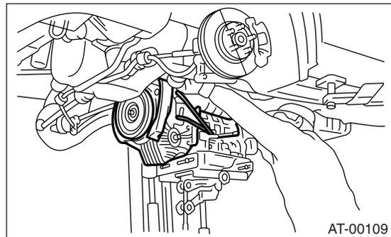
35) Separate the transmission assembly and rear cushion rubber.
