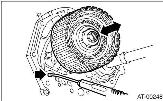
(9) Measure and record the clearance "B" between the retaining plate and snap ring. (Reverse clutch)
