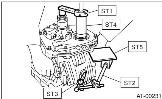
9) Adjust the tooth contact between front differential and drive shaft. <Ref. to 4AT-110, ADJUSTMENT, Drive Pinion Shaft Assembly.>
