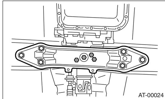
33) While gradually lowering the transmission jack, fully contact the engine support, and then tilt the engine rearward.
