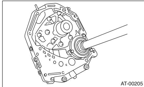
5) Rotate the drive pinion several times with ST1 and ST2.
