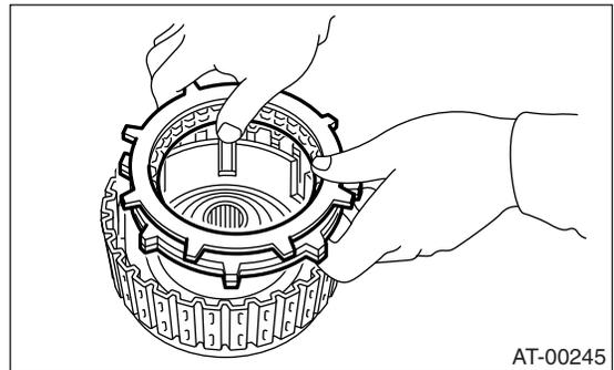
(2) Install snap ring to high clutch drum.
