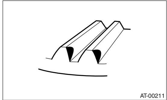
Corrective action: Increase thickness of drive pinion height adjusting washer in order to move drive pinion close to hypoid driven gear.
