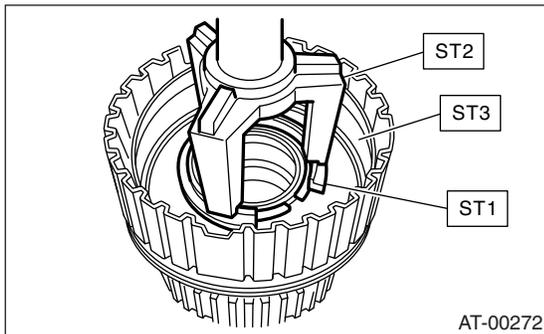
6) Install the dish plate, driven plates, drive plates, and retaining plate, and secure with the snap ring.
