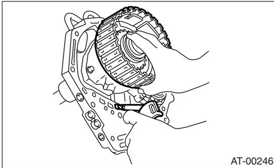
(10) Measure and record the clearance "B" between the retaining plate and snap ring. (High clutch)
