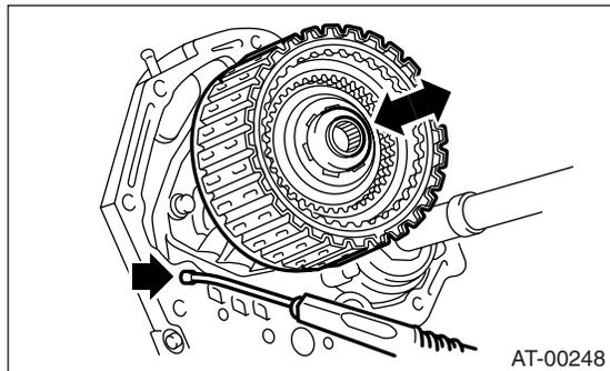
(3) Measure the clearance between the retaining plate and snap ring. (Reverse clutch) At this time, do not press down retaining plate.
