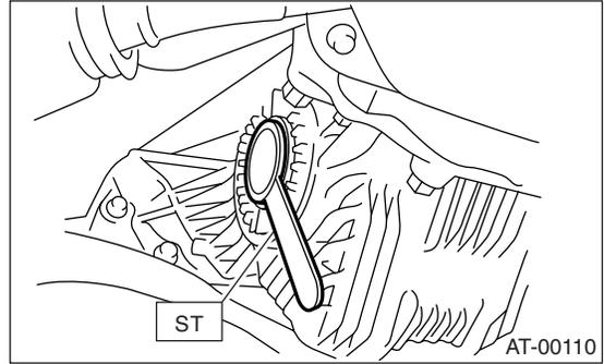
19) Align the spline of front differential shaft to that of differential bevel gear for insertion, and remove them using ST.
