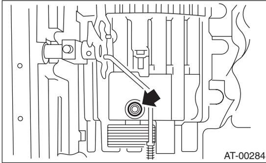
(3) After all 2-4 brake component parts have been installed, blow in air intermittently and confirm the operation of the brake.
