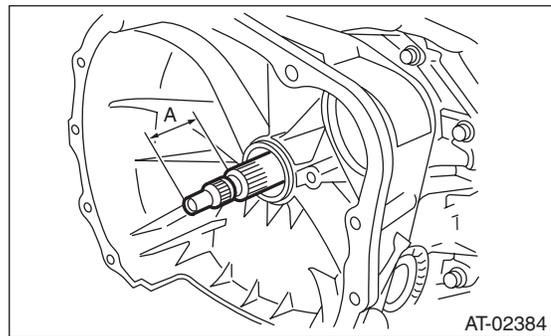
14) Install the torque converter clutch assembly. <Ref. to 4AT-81, INSTALLATION, Torque Converter Clutch Assembly.>
