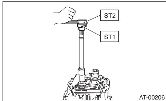
6) Tighten the LH retainer until contact is felt while rotating the shaft. Then loosen the RH retainer. Keep tightening the LH retainer and loosening the RH retainer until the pinion shaft can no longer be turned. This is the “zero” state.
