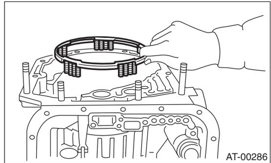
21) Remove the 2-4 brake piston and piston retainer without damaging.
