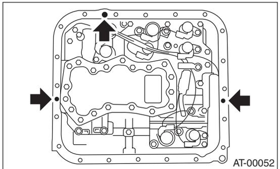
8) Install the oil pan with tightening bolts evenly.
