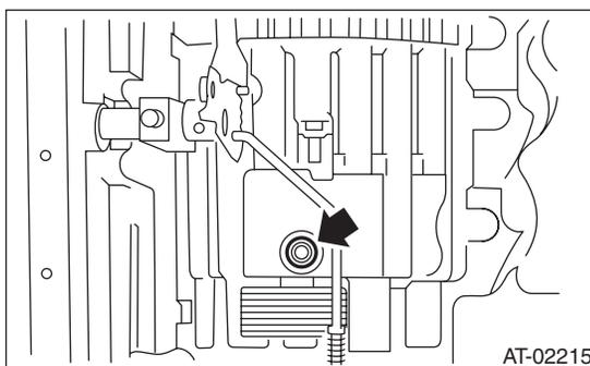
(9) After all 2-4 brake component parts have been installed, blow air intermittently and confirm the operation of brake.
