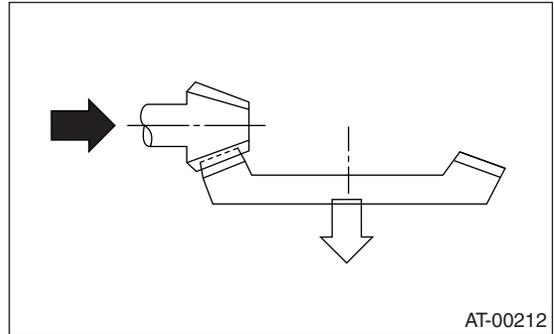
6) If tooth contact is correct, mark the retainer position and loosen it. After fitting a new O-ring and oil seal, screw in the retainer to the marked position. Then tighten the lock plate to the specified torque.
