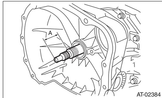
12) Install the torque converter clutch assembly. <Ref. to 4AT-81, INSTALLATION, Torque Converter Clutch Assembly.>
