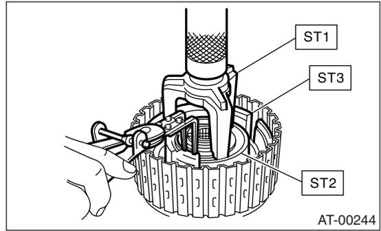
8) Selection of high clutch retaining plate (Turbo model)
