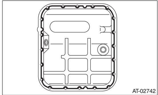
7) Apply liquid gasket fully to three holes other than screw holes on transmission case.
