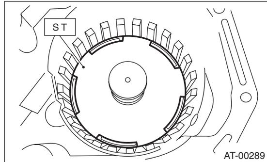
22) Install planetary gear and low clutch assembly to transmission case.
