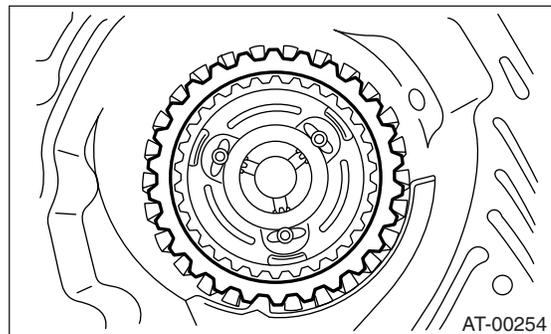
(2) Install a new 2-4 brake oil seal to transmission case.
