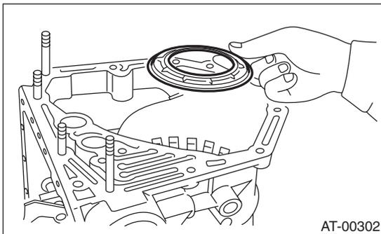
4) Install the one-way clutch inner race, spring retainer and return spring.
