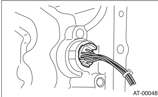
2) Connect the harness connectors. Connect the connectors of same color, and secure the connectors to valve body using clips. (Turbo model)
