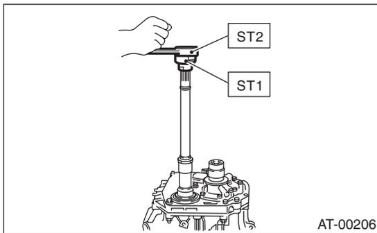
4) Adjust the backlash between drive pinion and hypoid driven gear. <Ref. to 4AT-117, ADJUSTMENT, Front Differential Assembly.>
