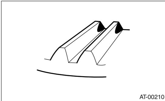
Corrective action: Decrease thickness of drive pinion height adjusting washer in order to move drive pinion away from hypoid driven gear.
