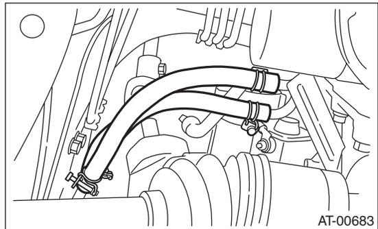
4) Connect ATF cooler hose to pipe of radiator side.
