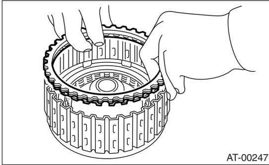
(8) Apply compressed air intermittently to check for operation.
