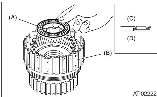
(A) Thrust needle bearing
