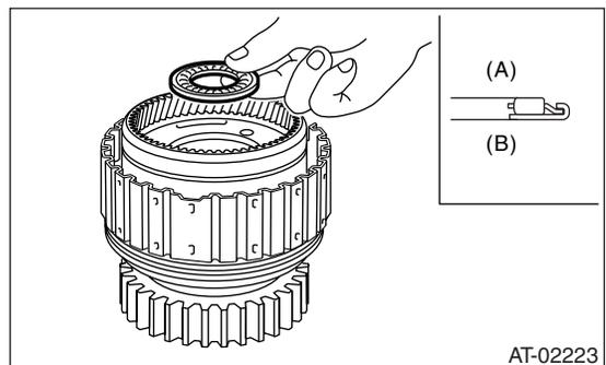
15) Install the rear sun gear in proper direction.
