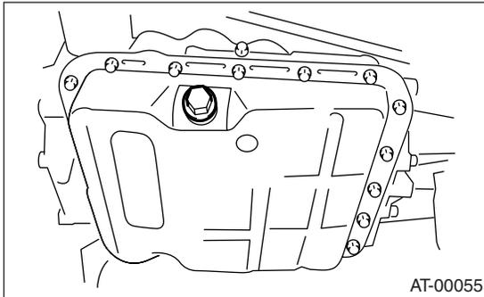
6) Replace the gasket with a new one, and then tighten the drain plug.
