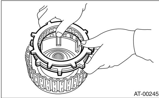
(8) Install the snap ring to high clutch drum.
