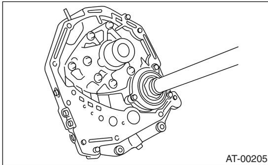
3) Rotate the drive pinion several times with ST1 and ST2.
