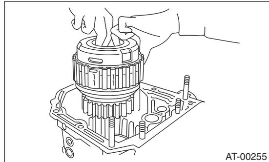
23) Selection of 2-4 brake retaining plate (Turbo model)
