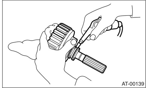
9) Check clearance between snap ring and pressure plate. <Ref. to 4AT-89, INSPECTION, Transfer Clutch.>
