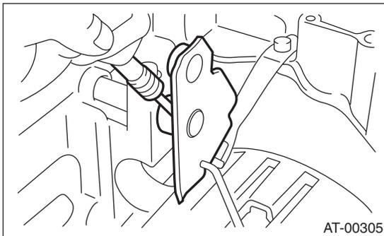
5) Install control valve assembly and oil pan. <Ref. to 4AT-62, INSTALLATION, Control Valve Body.>
