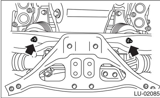
15) Remove the bolts which install the oil pan on cylinder block while raising up engine.
