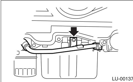
5) Remove the water pipe and hoses between oil cooler and water pump.
