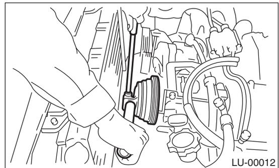
11) Remove the water pump. <Ref. to CO(H4DOTC)-19, REMOVAL, Water Pump.>
