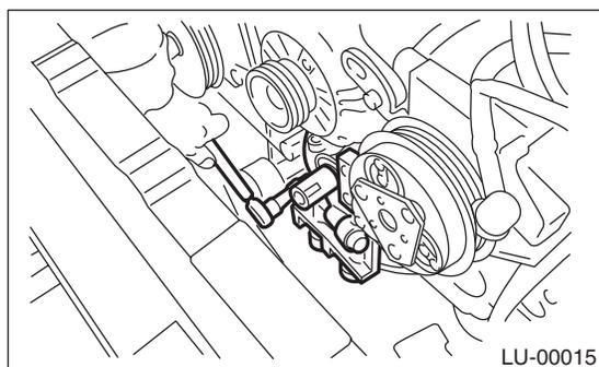
15) Remove the oil pump using flat tip screwdriver.
