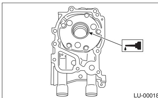
4) Be careful not to scratch the oil seal when installing the oil pump on cylinder block.
