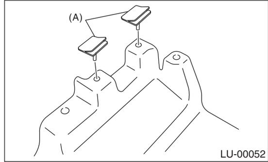
2) Install the baffle plate.
