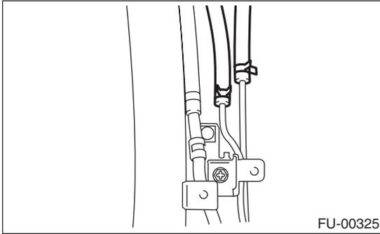
6) Insert the fuel filler hose (A) approx. 35 to 40 mm (1.38 to 1.57 in) over the lower end of fuel filler pipe, and then tighten the clamp.
