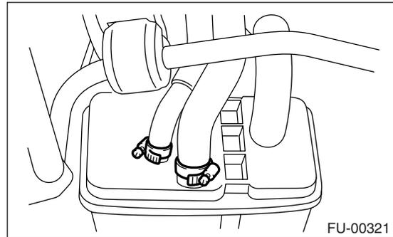
8) Tighten the band mounting bolts.
