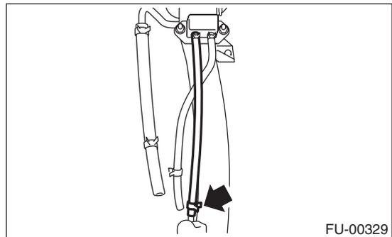
4) Install the evaporation pipe to the fuel filler pipe.
