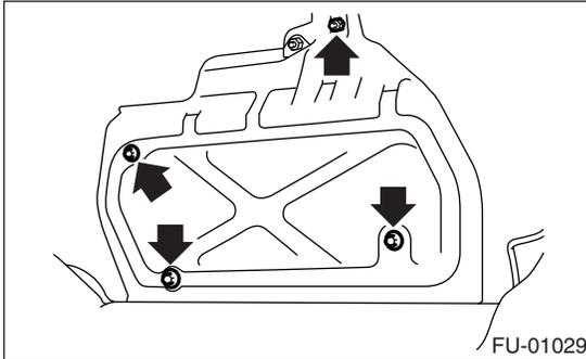
5) Remove the nuts (A) which hold ECM to the bracket.
