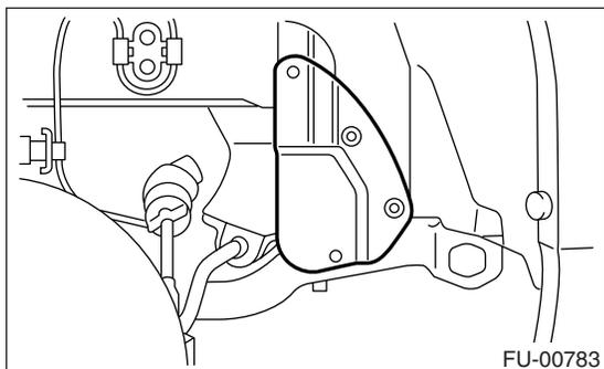
7) Apply spray type lubricant to the threaded portion of front oxygen (A/F) sensor, and leave it for one minute or more.
