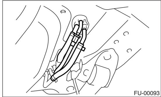
5) Connect the connector to the drain valve.
