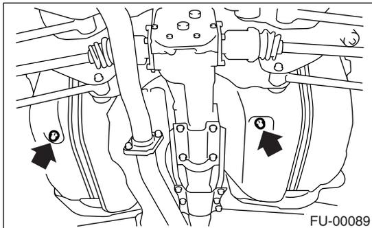
4) Tighten the fuel drain plug.
