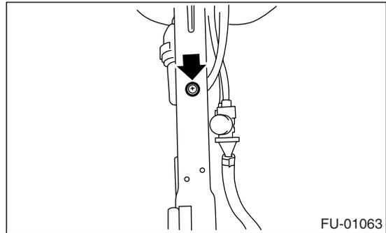
4) Separate the fuel filter from fuel pump.
