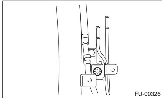
9) Tighten the bolts which hold evaporation hoses onto the clip of fuel filler pipe.
