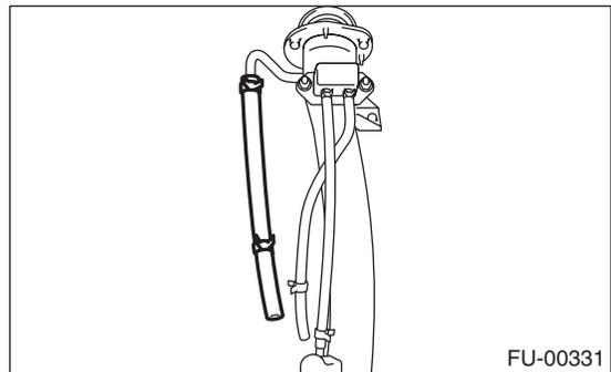
3) Connect the evaporation hose to the evaporation pipe.
