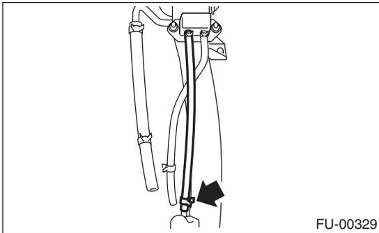
2) Remove the bolt which installs the joint pipe on fuel filler pipe.
