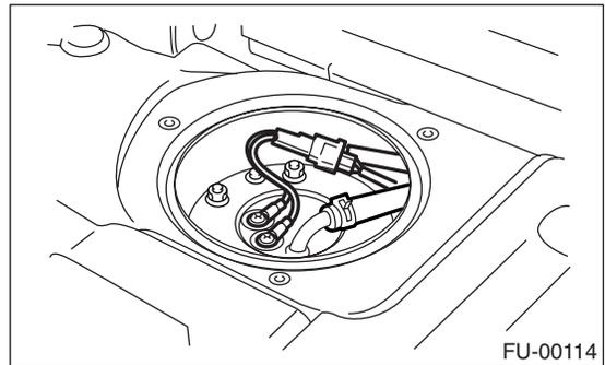
9) Remove the bolts which install the fuel sub level sensor on fuel tank.
