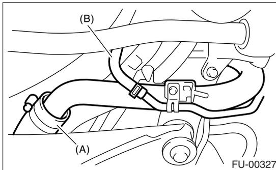
7) Insert the air vent hose approx. 25 to 30 mm (0.98 to 1.18 in) into the lower end of air vent pipe, and then hold the clip.
