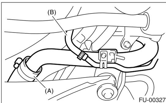
4) Connect the fuel hoses, and hold them with clips and quick connector. <Ref. to FU(STi)-62, INSTALLATION, Fuel Delivery, Return and Evaporation Lines.>
