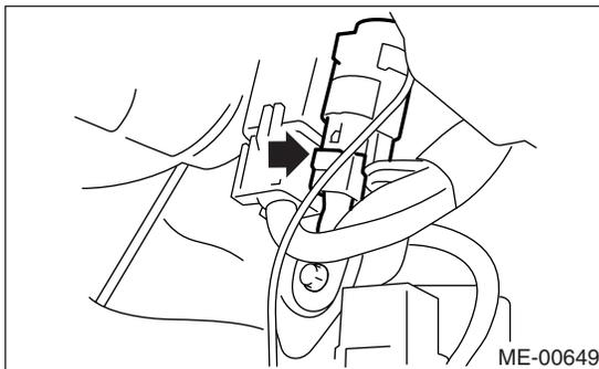
5) Remove the fuel pump relay from the mounting bracket.
