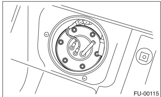
10) Remove the fuel sub level sensor.
