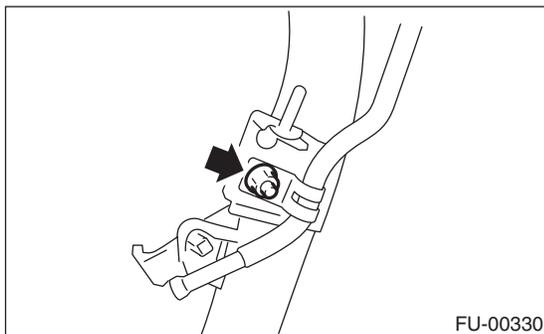
3) Disconnect the evaporation hose from the fuel filler pipe.
