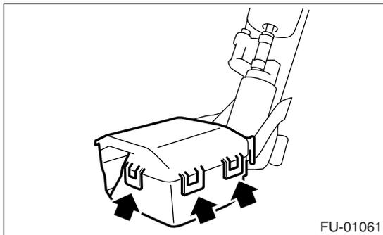
2) Disconnect the connector of fuel pump.
