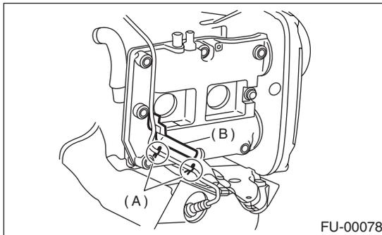
7) Connect the connector of front oxygen (A/F) sensor.
