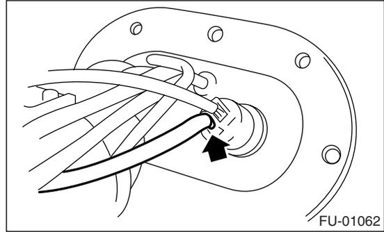
3) Remove the screw and remove the fuel pump and fuel filter.
