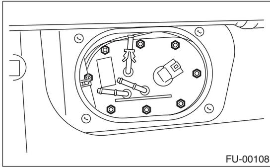
13) Take off the fuel pump assembly from the fuel tank.
