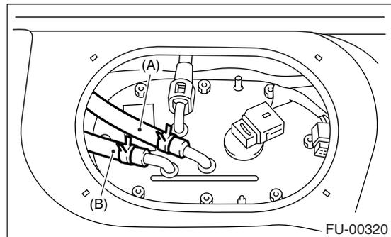
12) Remove the nuts which install the fuel pump assembly onto fuel tank.
