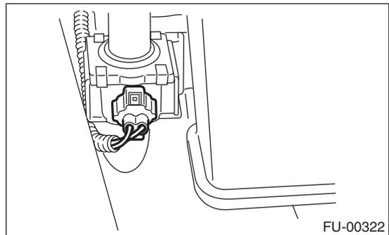
6) Connect the connector to the pressure control solenoid valve.
