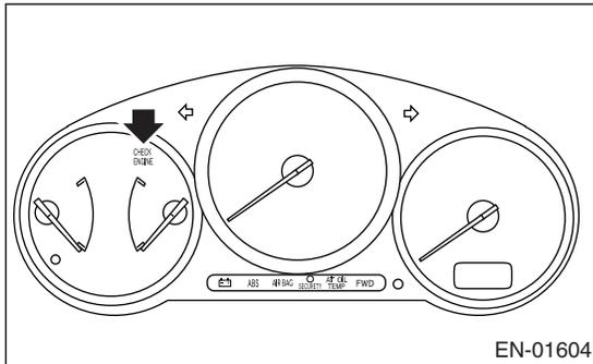
2) After starting the engine, the malfunction indicator light goes out. If it does not, either the engine or the emission control system is malfunctioning.
