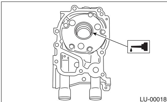
4) Be careful not to scratch the oil seal when installing oil pump on cylinder block.
