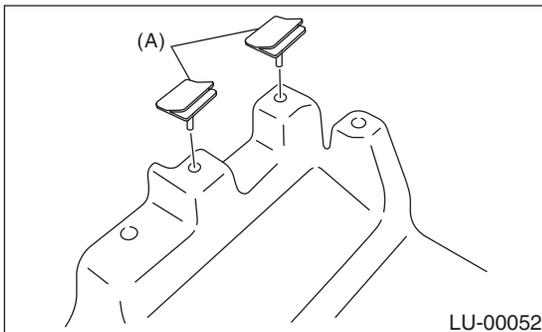
2) Install the baffle plate.
