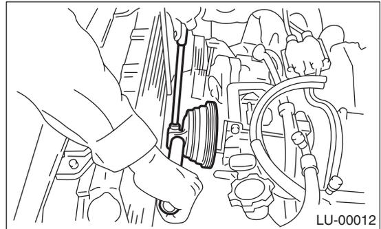
10) Remove the water pump. <Ref. to CO(H4SO)-14, REMOVAL, Water Pump.>
