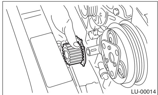
13) Remove the bolts which install the oil pump onto cylinder block.
