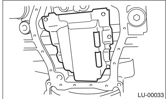
3) Install the oil strainer onto baffle plate.
