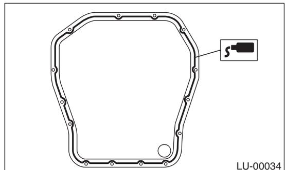
5) Tighten the bolts which install the oil pan onto engine block.
