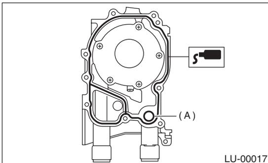
3) Apply a coat of engine oil to the inside of oil seal.
