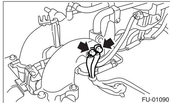
10) Use TCM mounting stud bolts at the body side grounding point when measuring voltage and resistance inside the passenger compartment.
