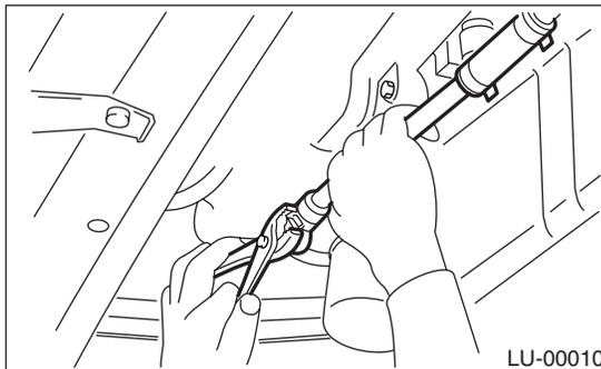
6) Remove the radiator. <Ref. to CO(H4SO)-18, REMOVAL, Radiator.>
