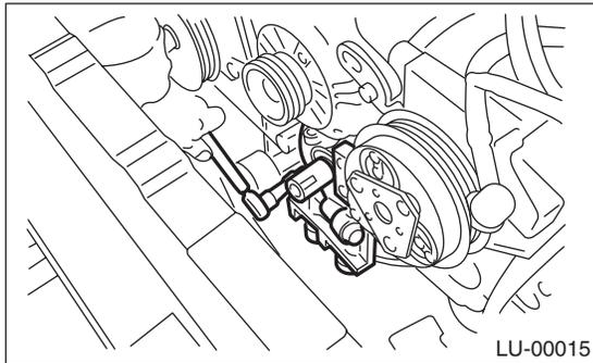
15) Remove the oil pump using the flat tip screwdriver.
