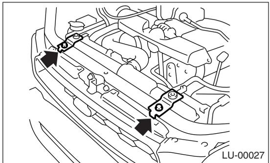
14) Install the intercooler. <Ref. to IN(H4DOTC)-10, INSTALLATION, Intercooler.>
