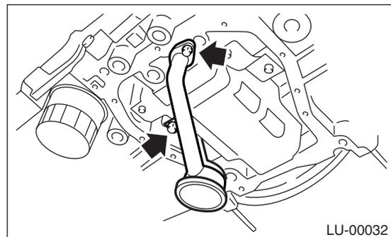
4) Apply liquid gasket to the mating surfaces, and then install the oil pan.
