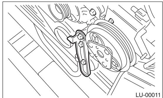
10) Remove the crank pulley by using ST.
