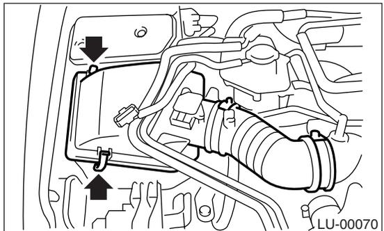
16) Connect the connector to mass air flow sensor.
