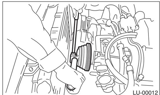
11) Remove the water pump. <Ref. to CO(H4SO)-14, REMOVAL, Water Pump.>
