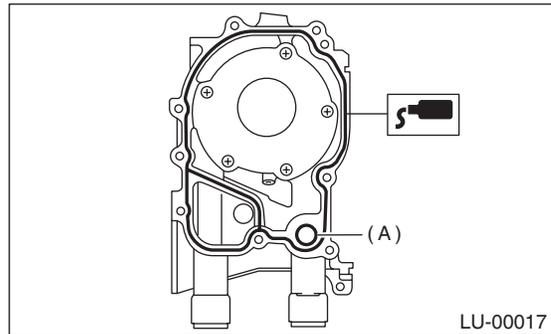
2) Replace the O-ring (A) with a new one.
