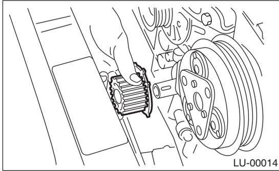
14) Remove the bolts which install the oil pump onto cylinder block.
