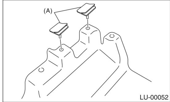
2) Install the baffle plate.
