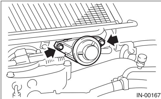
3) Remove the bolts which secure the intercooler to bracket.
