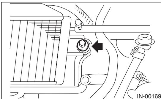
4) Remove the intercooler air duct from turbocharger.
