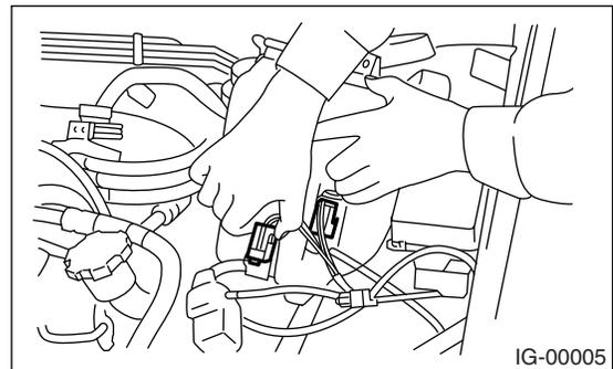
3) Disconnect the rear window glass washer hose from washer motor, then plug connection with a suitable cap.
