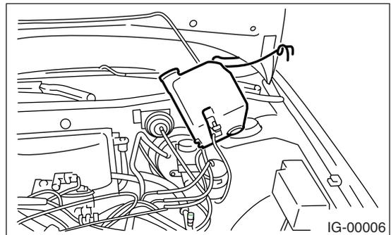
5) Disconnect the connector from ignition coil.
