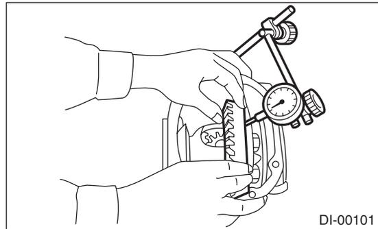
17) Checking and adjusting tooth contact of hypoid driven gear
