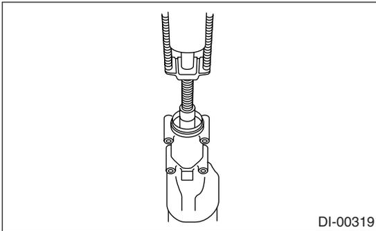
4) Pinion height adjusting washer selection.
