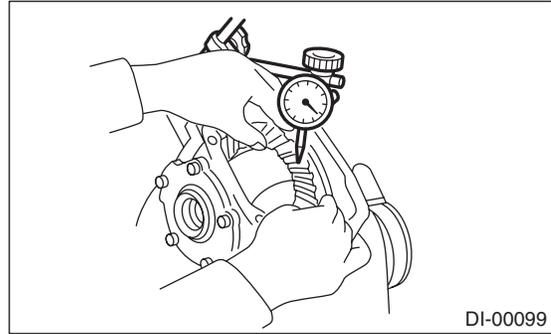
16) Check the hypoid driven gear runout on its back surface, and make sure that pinion and hypoid driven gear rotate smoothly.
