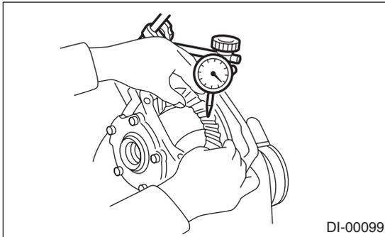
(7) At the same time, measure the total preload of drive pinion. Compared with the resistance when differential case is not installed, if the total preload is not within specification, adjust the thickness of side bearing retainer shims, increasing/reducing by an even amount at a time.
