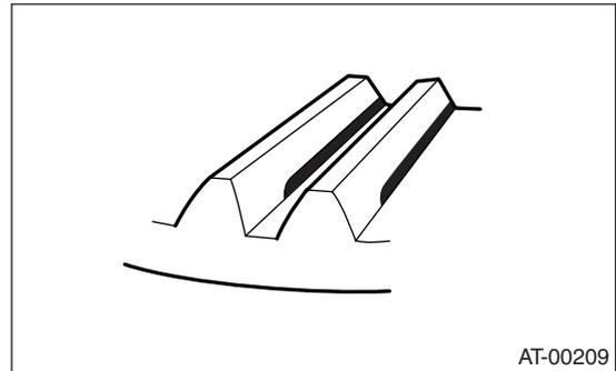
Corrective action: Reduce thickness of drive pinion height adjusting washer in order to move drive pinion away from hypoid driven gear.
