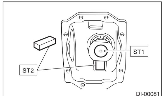
Drive pinion bearing preload
