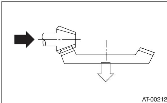
18) If proper tooth contact is not obtained, once again adjust the drive pinion height by changing RH and LH side bearing retainer shims and the hypoid gear backlash.
