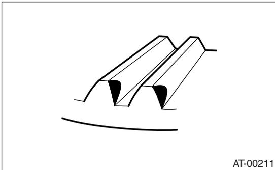
Corrective action: Increase thickness of drive pinion height adjusting washer in order to bring drive pinion close to hypoid driven gear.
