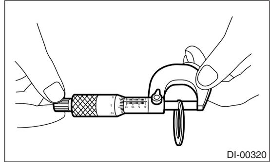
(2) Read the punch mark of installed drive pinion gear and new one.
