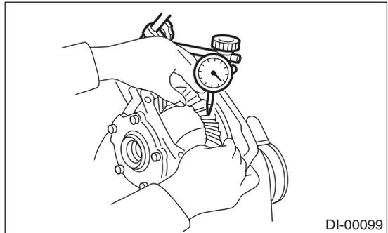
22) Check the hypoid driven gear runout on its back surface, and make sure that pinion and hypoid driven gear rotate smoothly.
