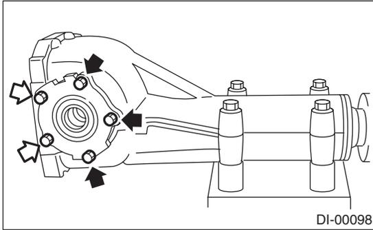
(6) Measure the hypoid driven gear-to-drive pinion backlash. Set the magnet base on differential carrier. Align the contact point of dial gauge with tooth face of hypoid driven gear, and move the hypoid driven gear while holding drive pinion still. Read the value indicated on dial gauge.
