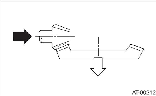
24) If proper tooth contact is not obtained, once again adjust the drive pinion height by changing RH and LH side bearing retainer shims and the hypoid gear backlash.
