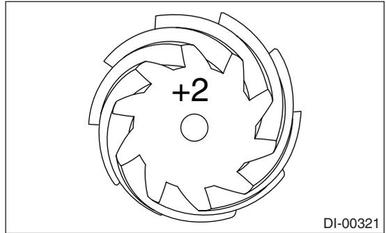
(3) Obtain the thickness of pinion height adjust shim to be inserted from the following formula, and replace the inserted shim with this one.
