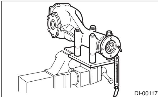
11) If bearing preload is out of specification, adjust to specification by selecting preload adjusting washer and spacer from the following table.
