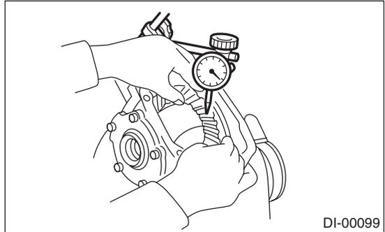
(7) At the same time, measure the total preload of drive pinion. Compared with the resistance when differential case is not installed, if the total preload is not within the specified range, readjust side bearing retainer shims, increasing/reducing by an even amount at a time.
